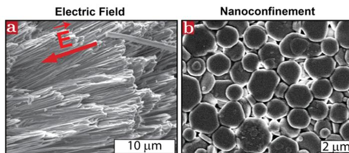
Figure 1. (a) The alignment boron nitride (BN) nanowires via an electric field. (b) The organization of BN nanoplates via nano-confinement.
