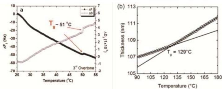
Figure 1. LbL  $T_g$ 's measured via (a) QCM-D and (b) temperature-controlled ellipsometry.
