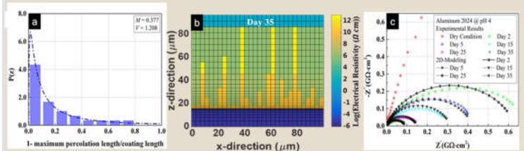
The electrochemical impedance response with time-dependent solution penetrations for degradation mechanism: a) Log-normal probability density function for the pore network distribution, b) The distribution of electrical resistivity at the 35<sup>th</sup> immersion day, c) Nyquist diagram.
