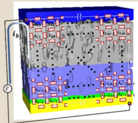
The schematic of 2D networks of electrochemical impedance elements for layer-by-layer composite coating system based on charge and energy conservation
