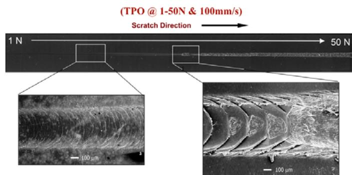
Figure 2. ASTM and ISO standardized scratch test applies linearly increasing load along surface, allowing the individual scratch mechanisms to be studied.
