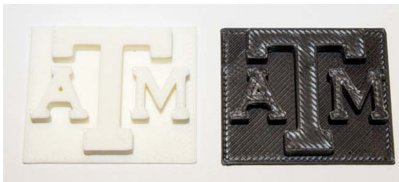
3D-printed structures without and with carbon nanotubes present
