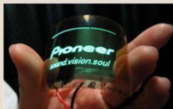
Figure 3: (a) Luminescence of an organic light-emitting diode deposited onto a flexible, low-CTE and optically transparent wood-cellulose nanocomposite. 13 (b) Mitsubishi Pencil's ballpoint pen, Uni-Ball Signo 307, with ink using CNF as a thickening agent (courtesy of Mitsubishi Pencil).
