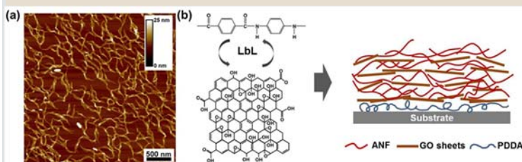
Figure. (a) An atomic force microscopy of solution-cast aramid nanofibers (ANFs). (b) Schematic of layer-by-layer (LbL) assembly of ANFs with graphene oxide (GO). (c) Schematic of final LbL composite containing ANFs, GO, and a polyelectrolyte (PDAA). Images adapted from ref. 5.
