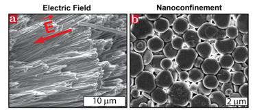
Figure 1. (a) The alignment boron nitride (BN) nanowires via an electric field. (b) The organization of BN nanoplates via nano-confinement.
