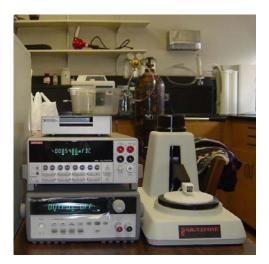
A four-point probe (FPP) has been built to measure sheet resistance and bulk resistivity of materials. Films with sheet resistance between 3000 and 0.01  $\Omega/\Box$  can be accurately measured. This system is currently being used to test electrically conductive polymer composites made with carbon black and carbon nanotubes.
