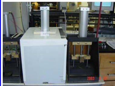
Figure 1 Custom-built creep station for adhesive specimen and environmental chambers.
