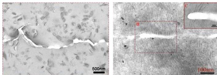
Figure 3. Crack propagation in ZrP-reinforced epoxy. On left, ZrP are partially exfoliated and crack propagates through rupture of clay tactoids. On right, individual ZrP do not interfere with the crack propagation and therefore do not affect fracture toughness of composite.
