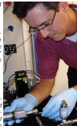
Dr. Shantz installs a membrane that will be tested for separating carbon dioxide and nitrogen as part of a Dow Chemical supported project.
