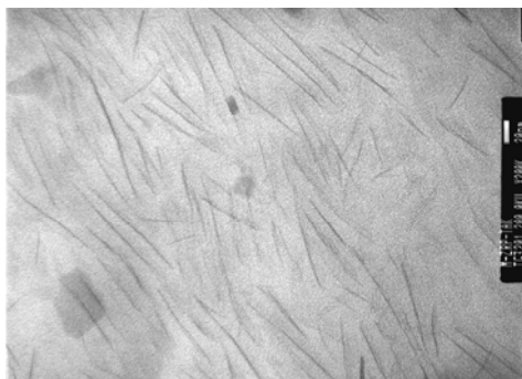
Fig. 2. TEM of zirconium phosphate-epoxy polymer nanocomposite showing the dispersion of layers in the polymer.
