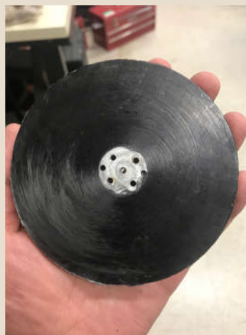
This model flywheel will combine carbon nanofiber with conventional carbon fiber to increase the energy storage density for home and industrial applications.
