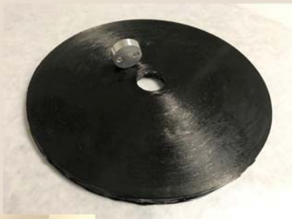
This flywheel is a hybrid containing convention commercial microfiber and high strength carbon nanofiber created in Dr. Mohammad Naraghi's laboratory.
